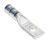
Penn-Union BLUA series compression lug, standard barrel, tinplated aluminum, 35 kV, 1/4in mounting bolt, 1-hole, 6 AWG, gray markings, AL9CU.
