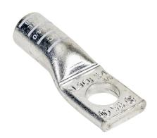
Penn-Union BLUA series compression lug, standard barrel, tinplated aluminum, 35 kV, 5/8in mounting bolt, 1-hole, 4/0 AWG, white markings, AL9CU.
