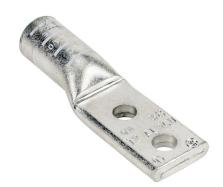
Penn-Union BLUA series compression lug, standard barrel, tinplated aluminum, 35 kV, 3/8in mounting bolt, 2-hole, 4/0 AWG, white markings, AL9CU.
