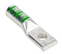
Penn-Union BLUA series compression lug, standard barrel, tinplated aluminum, 35 kV, 1/4in mounting bolt, 1-hole, 4 AWG, green markings, AL9CU.
