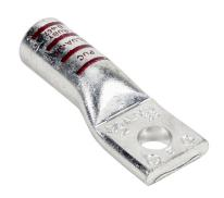
Penn-Union BLUA series compression lug, standard barrel, tinplated aluminum, 35 kV, 3/8in mounting bolt, 1-hole, 3/0 AWG, ruby markings, AL9CU.
