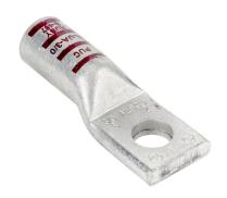
Penn-Union BLUA series compression lug, standard barrel, tinplated aluminum, 35 kV, 1/2in mounting bolt, 1-hole, 3/0 AWG, ruby markings, AL9CU.
