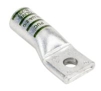
Penn-Union BLUA series compression lug, standard barrel, tinplated aluminum, 35 kV, 5/16in mounting bolt, 1-hole, 2/0 AWG, olive markings, AL9CU.
