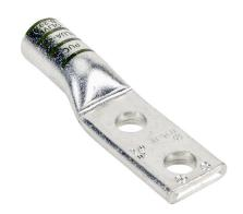
Penn-Union BLUA series compression lug, standard barrel, tinplated aluminum, 35 kV, 3/8in mounting bolt, 2-hole, 2/0 AWG, olive markings, AL9CU.
