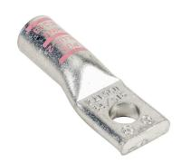
Penn-Union BLUA series compression lug, standard barrel, tinplated aluminum, 35 kV, 5/16in mounting bolt, 1-hole, 2 AWG, pink markings, AL9CU.
