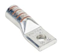
Penn-Union BLUA series compression lug, standard barrel, tinplated aluminum, 35 kV, 5/16in mounting bolt, 1-hole, 1/0 AWG, tan markings, AL9CU.
