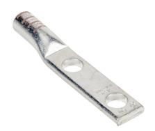
Penn-Union BLUA series compression lug, standard barrel, tinplated aluminum, 35 kV, 1/2in mounting bolt, 2-hole, 1/0 AWG, tan markings, AL9CU.
