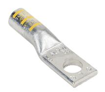
Penn-Union BLUA series compression lug, standard barrel, tinplated aluminum, 35 kV, 3/8in mounting bolt, 1-hole, 1 AWG, gold markings, AL9CU.
