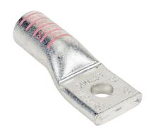
Penn-Union BLUA series compression lug, standard barrel, tinplated aluminum, 35 kV, 5/8in mounting bolt, 1-hole, 500 MCM, pink markings, AL9CU.
