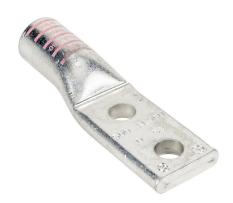
Penn-Union BLUA series compression lug, standard barrel, tinplated aluminum, 35 kV, 5/8in mounting bolt, 2-hole, 500 MCM, pink markings, AL9CU.
