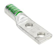
Penn-Union BLUA series compression lug, standard barrel, tinplated aluminum, 35 kV, 5/8in mounting bolt, 2-hole, 400 MCM, green markings, AL9CU.
