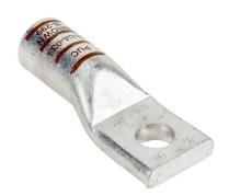
Penn-Union BLUA series compression lug, standard barrel, tinplated aluminum, 35 kV, 5/8in mounting bolt, 1-hole, 350 MCM, brown markings, AL9CU.
