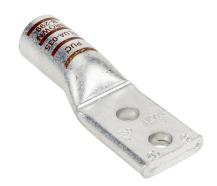
Penn-Union BLUA series compression lug, standard barrel, tinplated aluminum, 35 kV, 3/8in mounting bolt, 2-hole, 350 MCM, brown markings, AL9CU.
