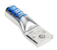
Penn-Union BLUA series compression lug, standard barrel, tinplated aluminum, 35 kV, 3/8in mounting bolt, 1-hole, 300 MCM, blue markings, AL9CU.
