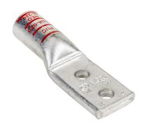
Penn-Union BLUA series compression lug, standard barrel, tinplated aluminum, 35 kV, 3/8in mounting bolt, 2-hole, 250 MCM, red markings, AL9CU.
