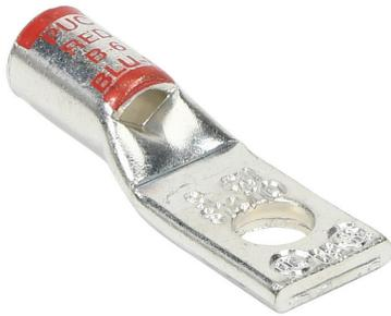
Penn-Union BLU series compression lug, standard barrel, tin-plated copper, 35 kV, #10 mounting bolt, 1 hole, 8 AWG, red markings.
