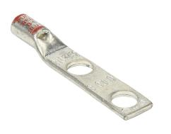
Penn-Union BLU series compression lug, standard barrel, tinplated copper, 35 kV, 1/4in mounting bolt, 2 hole, 0.75in hole spacing, 8 AWG, red markings.
