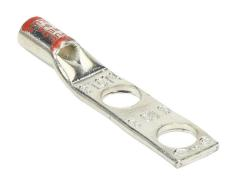
Penn-Union BLU series compression lug, standard barrel, tinplated copper, 35 kV, 1/4in mounting bolt, 2 hole, 0.63in hole spacing, 8 AWG, red markings.
