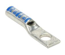
Penn-Union BLU series compression lug, standard barrel, tinplated copper, 35 kV, 1/4in mounting bolt, 1 hole, 6 AWG, blue markings.
