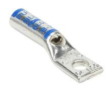
Penn-Union BLU series compression lug, standard barrel, tinplated copper, 35 kV, #10 mounting bolt, 1 hole, 6 AWG, blue markings.
