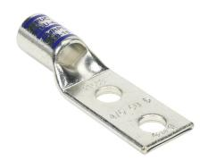
Penn-Union BLU series compression lug, standard barrel, tinplated copper, 35 kV, 3/8in mounting bolt, 2 hole, 1in hole spacing, 4/0 AWG, purple markings.
