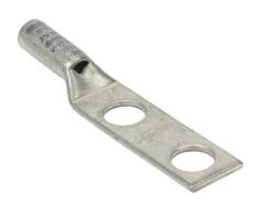
Penn-Union BLU series compression lug, standard barrel, tinplated copper, 35 kV, 3/8in mounting bolt, 2 hole, 1in hole spacing, 4 AWG, gray markings.
