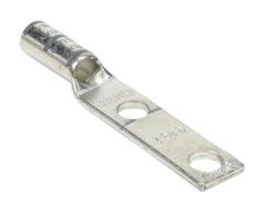
Penn-Union BLU series compression lug, standard barrel, tinplated copper, 35 kV, 1/4in mounting bolt, 2 hole, 1in hole spacing, 4 AWG, gray markings.
