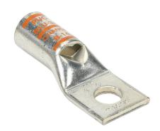
Penn-Union BLU series compression lug, standard barrel, tinplated copper, 35 kV, 3/8in mounting bolt, 1 hole, 3/0 AWG, orange markings.
