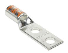
Penn-Union BLU series compression lug, standard barrel, tinplated copper, 35 kV, 3/8in mounting bolt, 2 hole, 1in hole spacing, 3/0 AWG, orange markings.
