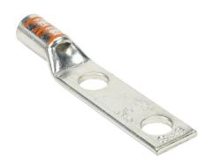
Penn-Union BLU series compression lug, standard barrel, tinplated copper, 35 kV, 1/2in mounting bolt, 2 hole, 1.75in hole spacing, 3/0 AWG, orange markings.
