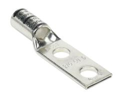
Penn-Union BLU series compression lug, standard barrel, tinplated copper, 35 kV, 3/8in mounting bolt, 2 hole, 1in hole spacing, 2/0 AWG, black markings.
