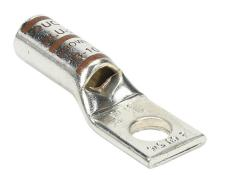
Penn-Union BLU series compression lug, standard barrel, tinplated copper, 35 kV, 5/16in mounting bolt, 1 hole, 2 AWG, brown markings.
