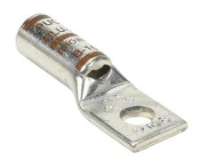
Penn-Union BLU series compression lug, standard barrel, tinplated copper, 35 kV, 1/4in mounting bolt, 1 hole, 2 AWG, brown markings.
