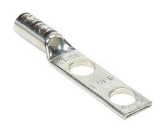
Penn-Union BLU series compression lug, standard barrel, tinplated copper, 35 kV, 3/8in mounting bolt, 2 hole, 1in hole spacing, 2 AWG, brown markings.
