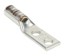
Penn-Union BLU series compression lug, standard barrel, tinplated copper, 35 kV, 1/4in mounting bolt, 2 hole, 0.63in hole spacing, 2 AWG, brown markings.
