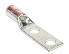
Penn-Union BLU series compression lug, standard barrel, tinplated copper, 35 kV, 3/8in mounting bolt, 2 hole, 1in hole spacing, 1/0 AWG, pink markings.
