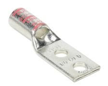
Penn-Union BLU series compression lug, standard barrel, tinplated copper, 35 kV, 1/4in mounting bolt, 2 hole, 0.63in hole spacing, 1/0 AWG, pink markings.
