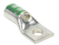
Penn-Union BLU series compression lug, standard barrel, tinplated copper, 35 kV, 1/4in mounting bolt, 1 hole, 1 AWG, green markings.
