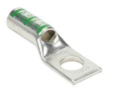
Penn-Union BLU series compression lug, standard barrel, tinplated copper, 35 kV, 3/8in mounting bolt, 1 hole, 1 AWG, green markings.
