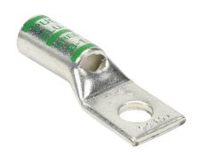
Penn-Union BLU series compression lug, standard barrel, tinplated copper, 35 kV, 5/16in mounting bolt, 1 hole, 1 AWG, green markings.
