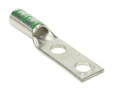
Penn-Union BLU series compression lug, standard barrel, tinplated copper, 35 kV, 5/16in mounting bolt, 2 hole, 0.88in hole spacing, 1 AWG, green markings.
