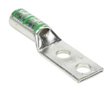
Penn-Union BLU series compression lug, standard barrel, tinplated copper, 35 kV, 1/4in mounting bolt, 2 hole, 0.63in hole spacing, 1 AWG, green markings.
