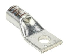
Penn-Union BLU series compression lug, standard barrel, tinplated copper, 35 kV, 5/8in mounting bolt, 1 hole, 500 MCM, brown markings.
