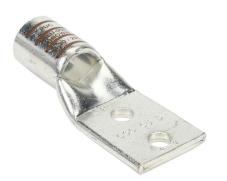
Penn-Union BLU series compression lug, standard barrel, tinplated copper, 35 kV, 3/8in mounting bolt, 2 hole, 1in hole spacing, 500 MCM, brown markings.
