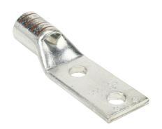
Penn-Union BLU series compression lug, standard barrel, tinplated copper, 35 kV, 1/2in mounting bolt, 2 hole, 1.75in hole spacing, 500 MCM, brown markings.
