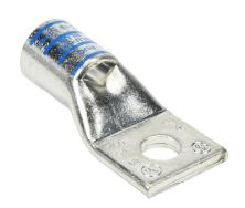
Penn-Union BLU series compression lug, standard barrel, tinplated copper, 35 kV, 1/2in mounting bolt, 1 hole, 400 MCM, blue markings.
