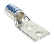
Penn-Union BLU series compression lug, standard barrel, tinplated copper, 35 kV, 3/8in mounting bolt, 2 hole, 1in hole spacing, 400 MCM, blue markings.
