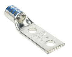
Penn-Union BLU series compression lug, standard barrel, tinplated copper, 35 kV, 1/2in mounting bolt, 2 hole, 1.75in hole spacing, 400 MCM, blue markings.
