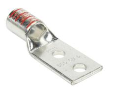
Penn-Union BLU series compression lug, standard barrel, tinplated copper, 35 kV, 3/8in mounting bolt, 2 hole, 1in hole spacing, 350 MCM, red markings.
