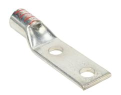
Penn-Union BLU series compression lug, standard barrel, tinplated copper, 35 kV, 1/2in mounting bolt, 2 hole, 1.75in hole spacing, 350 MCM, red markings.
